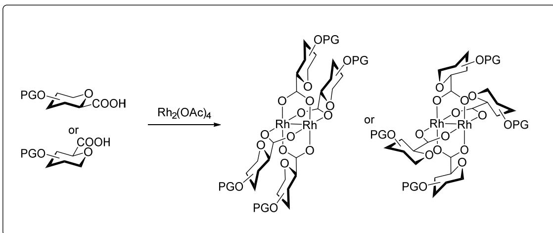
In this work, we present the synthesis of new carbohydrate derived rhodium carboxylate complexes as well as their application in enantioselective carbennoid cyclopropanation catalysis.
