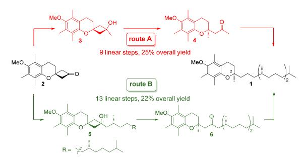
In an alternative approach (route B), the side chain was first introduced in a sequence of enyne metathesis and 1,4-hydrogenation.<sup>[2]</sup> After Pfaltz-hydrogenation of the resulting threefold-substituted olefin, the "late-stage" asymmetric Ir-catalyzed cyclobutanol opening proceeded with even better stereoselectivity to give ketone **6** (d.r. >99:1).
